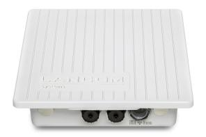
The LANCOM OAP-830 features two radio modules for parallel operation in the 2.4- and 5-GHz frequency bands. Integrated sector antennas make it ideal for high-performance, reliable hotspots, and also for outdoor enterprise applications.
