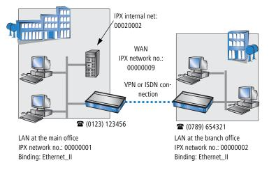
According to IPX convention, the three necessary network numbers are referred to as "external network numbers". Similar to IP network addresses, they apply for an entire LAN segment. Conversely, the IPX internal network numbers are for addressing a particular Novell server in the LAN. All three of these network numbers must differ not only from one another but also from all IPX internal network numbers being used.
