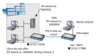
According to IPX convention, the necessary network numbers are referred to as "external network numbers". Similar to IP network addresses, they apply for an entire LAN segment. Conversely, the IPX internal network numbers are for addressing Novell servers in the LAN. All three of these network numbers must differ not only from one another but also from all IPX internal network numbers being used.
