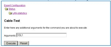
Change then to menu item **Expert configuration** ➤ **Status** ➤ **LAN statistics** ➤ **Cable test results**. The results of the cable test for the individual interfaces are show up in a list.
