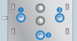
Wall mounting wall using the holes (1), (2) and (3).
