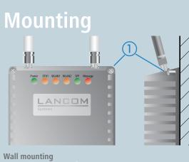
Using suitable screws (1), mount your device in the required position on the wall. Screws for wall mounting are not supplied with the device.
