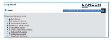
The settings are not stored in the device until inputs are confirmed on the last screen of the Wizard.
