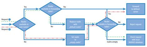
Using different realm tags allows different RADIUS servers to be targeted with requests. The way in which the LANCOM's RADIUS server makes decisions for the two requests is shown in the diagram.
