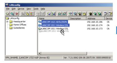
③ The 1-Click-VPN Site-to-Site Wizard will be started. Enter a name for this access and select the address under which the router is accessible from the Internet.
