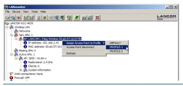
Assignment of the configuration causes the Access Point to be entered into the AP table in the WLAN Controller. It takes a few seconds for the WLAN Controller to assign a certificate to the Access Point and for this to become an active element in the central WLAN infrastructure.
