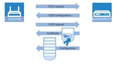
Authentication and configuration can both be carried out either automatically or only with a corresponding entry of the Access Point's MAC address in the AP table of the WLAN Controller. If the Access Point's WLAN modules were deactivated at the beginning of the DTLS communication, these will be activated after successful transfer of the certificate and configuration (provided they are not explicitly deactivated in the configuration).
