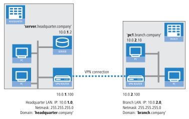
Unlike with Internet access, network connectivity makes all of IP addresses visible in all participating networks, including those in the remote LAN, and not just that of the router. The computer with the IP address 10.0.2.10 in the branch-office LAN sees the server 10.0.1.2 at the main office and, with the appropriate rights, has access to it. The same applies in the other direction.
