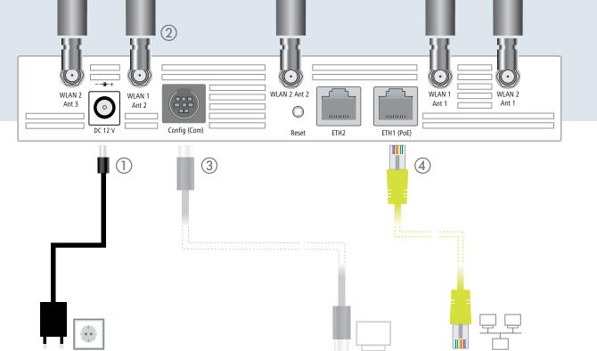
1 Power cable to the device, turn the bayonet connector 90° clockwise until it
