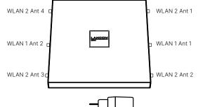
After connecting the cable to the device, turn the connector 90° clockwise to prevent it from accidental unplugging. Use only the supplied power adapter.
