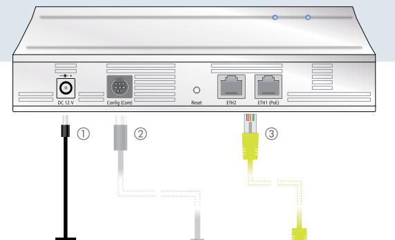
1 Power When connecting the cable to the device, turn the bayonet connector 90° clockwise.
