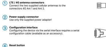
Pressed up to 5 seconds: device restart Pressed until first flashing up of all LEDs: configuration reset and device restart
