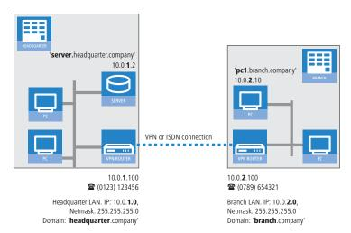
Unlike with Internet access, network connectivity makes all of IP addresses visible in all participating networks, including those in the remote LAN, and not just that of the router. The computer with the IP address 10.0.2.10 in the branch-office LAN sees the server 10.0.1.2 at the main office and, with the appropriate rights, has access to it. The same applies in the other direction.
