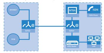
ADSL can operate over both ISDN- and analog telephone lines (POTS – **P**lain **O**ld **T**elephone **S**ervice). Devices with an integrated modem are supplied in two versions. Information about the supported telephone system is to be found on the type designation on the underside of the device. The device name is marked on the label along with a suffix which indicates the supported telephone system:
