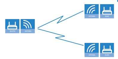
Thus it is recommended for the 5 GHz band that one central access point should be configured as 'Master' and all other point-to-point partners should be configured as 'Slave'. In the 2.4 GHz band, too, this setting simplifies the establishment of point-to-point connections if the automatic channel search is activated.
