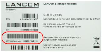
A device with the LAN MAC address "00A05713B178" thus has a preshared key of "L00A05713B178". This key is entered into the 'WPA or private WEP settings' of the device for each logical WLAN network as 'Key 1/Passphrase'.
