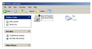
For checking the installation, click with the right mouse button on the fax-icon and select **Properties**. The LANCOM CAPI Faxmodem should now be entered into register 'devices'.
