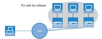
With LANCAPI by LANCOM it is possible to send faxes comfortably from your workstation PC, without having connected a fax device. To do so, you need to install several components:
